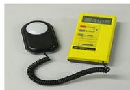
A lux meter for measuring illuminance in work places.
