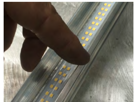
Close up of Narrow Beam Reflective optics installed on LED Strip in Extrusion
